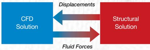
Implicit coupling for fluid structure interaction includes iterative analyses of fluid forces that may cause structural reactions, which in turn may alter fluid flow.
