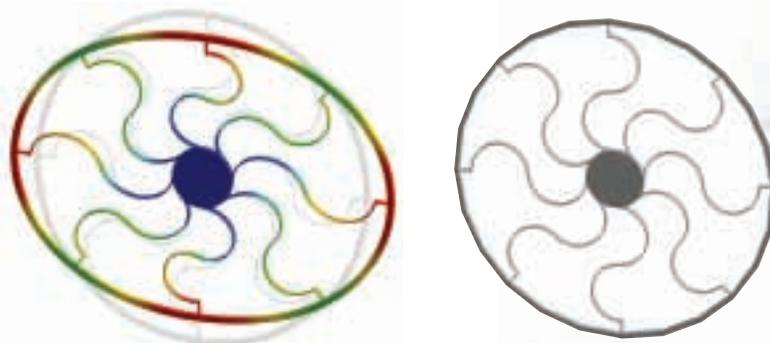
Analysis of the harmonic response of micromachined silicon ring gyroscope, including the effects of thermoelastic damping
