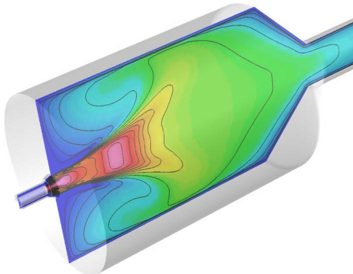
Temperature contour cross section through a natural gas burner
