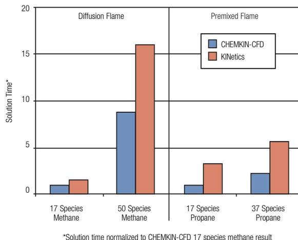
Improvements in solution time with the new CHEMKIN-CFD compared to the previous software version
