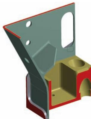
Submodel of high stress regions in ANSYS DesignModeler software. Cut boundaries are shown in red.
