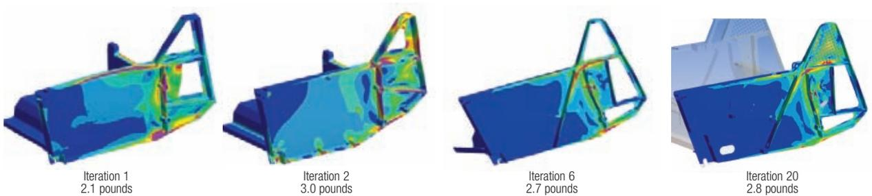
Equivalent stress plots from various iterations of the ACES 5 ejection seat bucket design. Weight of the bucket, one of the design considerations, is shown for each.
