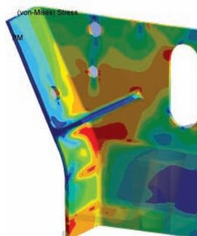
Submodel results provide more-accurate stress results than the global static model.
