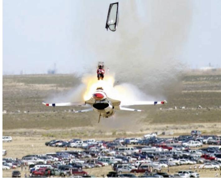
An ejection seat, used in emergency situations in military aircraft. An explosive charge or rocket motor thrusts the seat out of the aircraft, carrying the pilot with it. Once airborne, a parachute is deployed. This photo shows the ACES II ejection seat. U.S. Air Force photo by Staff Sgt. Bennie J. Davis III.
