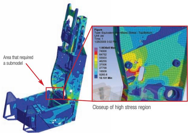
Stress loads that result from static analysis of ejection at aircraft speed of 750 mph
