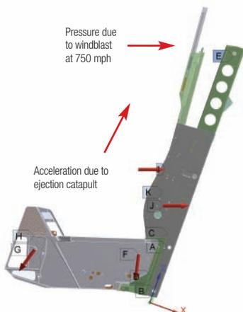
Loads imparted on the seat when ejected from an aircraft travelling at 750 mph
