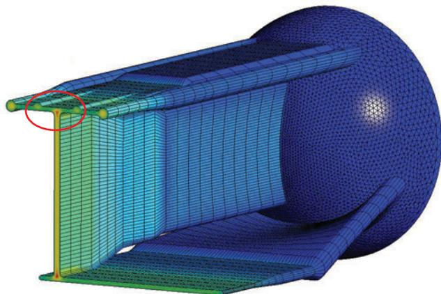
Simulation calculated outlet velocities for resin exiting the die. The highest velocity is shown in the circled area of the upper T-junction.
