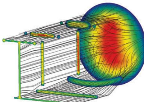
Simulation shows color-coded resin velocities and flow paths inside the length of the extrusion die, with uneven flow for the original die (left) and more balanced velocity distribution for the optimized design (right).
