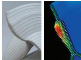
Validation of the simulation model (right) with an extruded part (left) shows good correlation. Note the bulge in the high-velocity region predicted by simulation.
