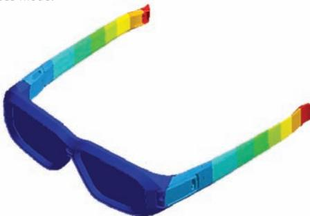
Deformation that occurs when worn by 95th percentile of males
