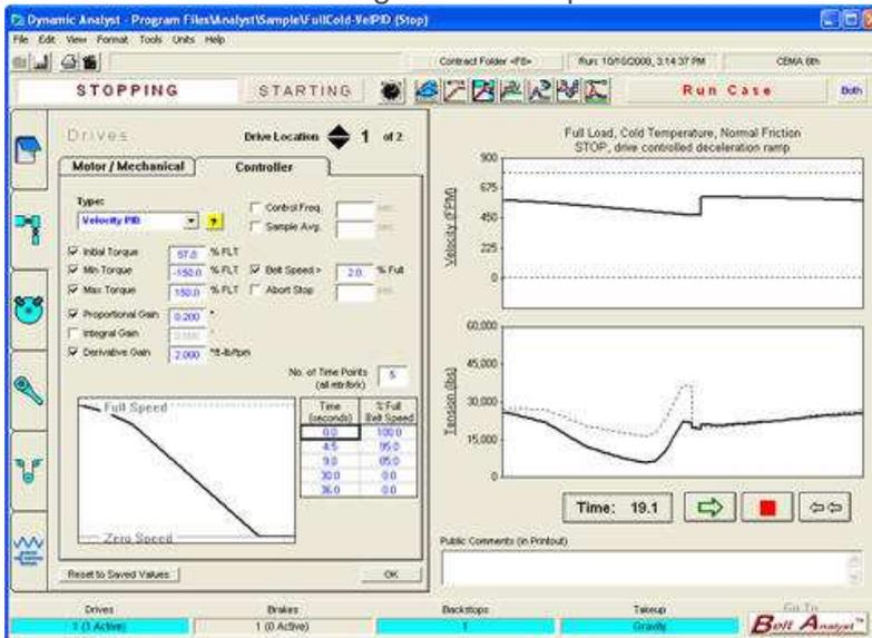
Watch an animation of the belt tensions and belt velocities change from full speed to stopped and back to full speed. There is no better way to understand the transient stress wave migration through the belt than with this specialized animation.
