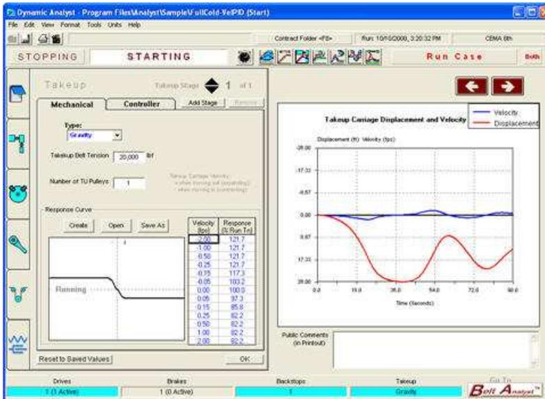
Stop your conveyor with brakes or the drives. Determine accurate dynamic loads on the holdbacks.
