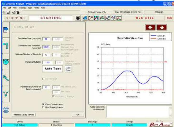
Perhaps the most useful feature that has made this advanced tool useable for all; Auto Tuning. FEA analysis is not easy to setup. But now the program does most of the work by automatically setting up damping factors, time steps and element sizes in the most efficient manner for all application.
