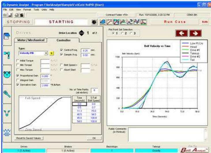
Easily model the starting characteristics of fluid couplings, reduced voltage starters, wound rotor induction motors with multiple resistance steps, hydro viscous clutch, VFD, DC or any other type of start. Define a velocity curve and PID loop parameters.
