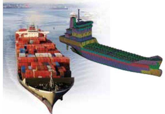
*“Ocean-going merchant ships are slammed by natural forces and loads generated by complex FSI. We use software from ANSYS at the start of the design process to identify vibration and other problems early on and make changes to get the design right the first time.”*
