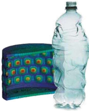
Design engineers work every day with materials, components and assemblies that inherently behave in nonlinear ways. Buckling presents itself as a large deformation, for example. Using our software to solve nonlinear problems improves the accuracy of results and ultimately results in better-designed products.
